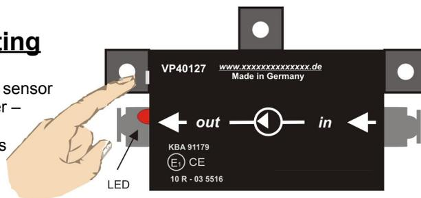
**Step 1:** Start the vehicle and activate gas operation. The dosing module is now provided with power and remains in Set-up ready mode (LED lights up yellow) for 30 seconds.
