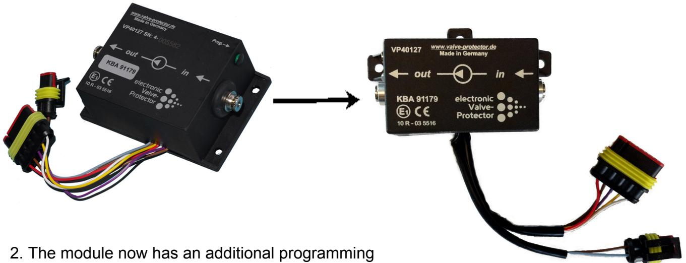
2. The module now has an additional programming method at your fingertips. This allows an adjustment of the Dosage without using a PC (see Progr. instructions in the appendix). The module can also be adjusted with the outstanding Valve Protector Software V3.x. When delivered, the use of finger-Progr. is unlocked. With the VP software, version 3.4.4, the use of fingertip programming be shut down
